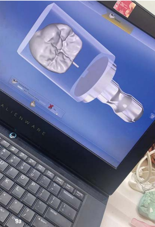
Figs. 9a–c: Creation of the CAD for the endocrown (a). Grandio blocs A3 LT block ready for milling (b). Endocrown milled from Grandio blocs (c).
